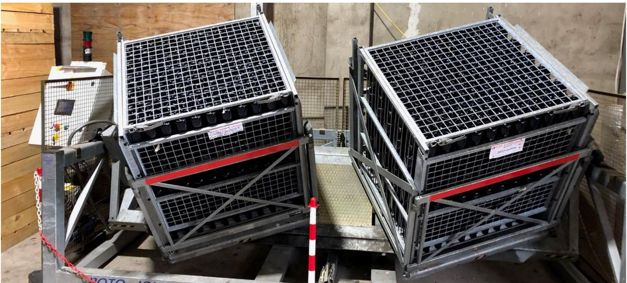
Once the bottles have been properly riddled, they can be disgorged. This is done in the cool room with the bottles chilled to 2°. The beer cap is removed and the pressure inside the bottle (approximately 6 bar, the same pressure as a bus tyre) blows out the yeast lees in a very impressive explosion! And this is the answer to the Christmas riddle!
